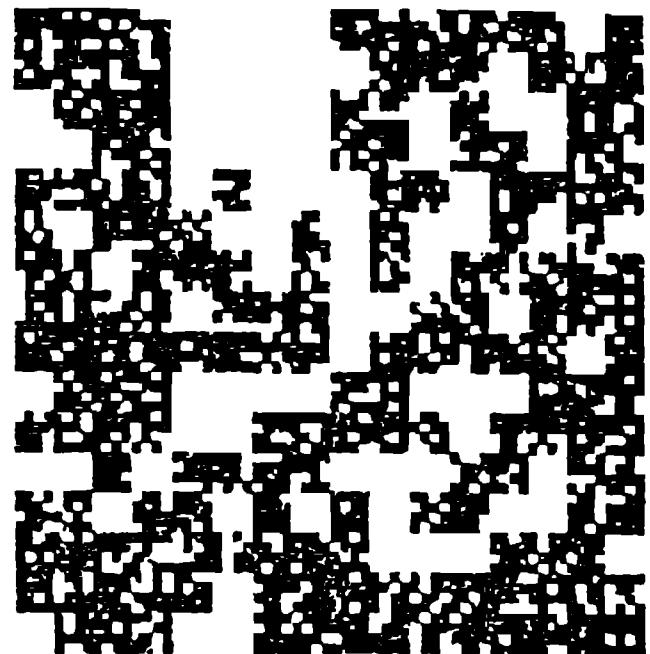
Fig. 5b. An example of a canonical β model in d = 2 with a 4 \times 4 breakup per cascade step, showing the first four steps; black indicates the remaining "alive" regions. Fractal dimension is set at D = 1.73 , i.e., at each step, each cell has a probability 4^{-0.27} = 0.688 \dots of remaining alive where 0.27 = C = 2 - D .
