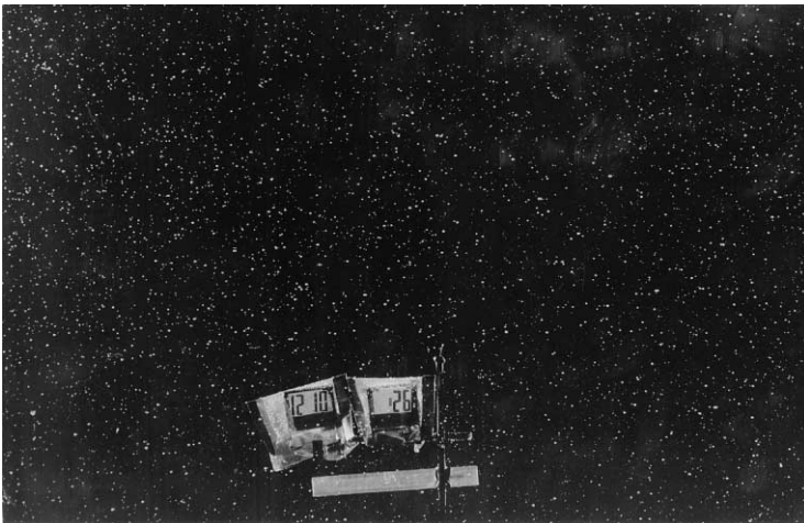
Fig. 10. Blown-up section of a photograph of a typical rain event, including the alarm clocks. The clocks were approximately 12 cm wide and were placed at the center of the region of interest.
