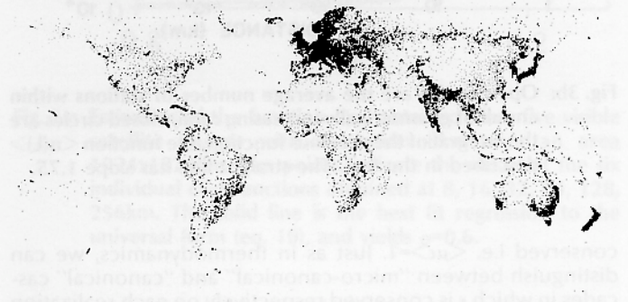
Fig. 3a: The locations of the 9,563 station in the global meteorological measuring network showing their high degree of sparseness (from Lovejoy et al 1986).
