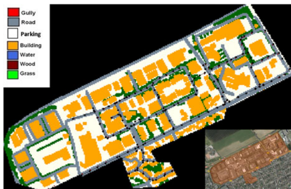
Figure 4. Map of the land use distribution inputted in Multi-Hydro for the Loup catchment with pixels of size 10\text{ m} \times 10\text{ m} . The sewer network modelled with SWMM is superposed to this map (the nodes and conduits are visible along most of the roads). Satellite image the catchment (lower right).
