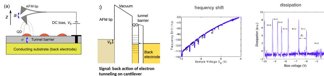
4.3. The microscope works at low temperature (4.5 K)
