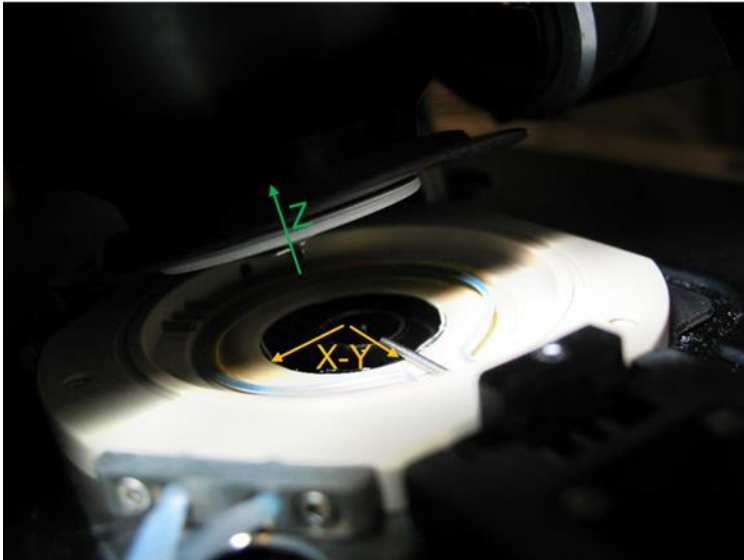
(FIGURE. 3.1.1) AFM HEAD AND SCHEMATICS SHOWING PIEZO ACTUATION SYSTEMS. THE USE OF THE LINEAR VARIABLE DIFFERENTIAL TRANSFORMER (LVDT) SUPPRESSES THE HYSTERESIS OF THE PIEZO MOTION AND REPORTS A MORE ACCURATE POSITION.
