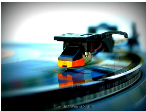
Figure. 1 Scanning Probe Microscopy Principle. This figures illustrate in (a) a vinyl record player needle converting the surface features into sound (image taken from Wingnut Designs), and (b) Schematic of AFM tip scanning across a surface sensing the variations in height over the atoms. Note SPM the probe scanned determines the magnitude measured.
