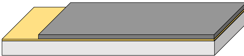
FIGURE 2.12: Schematic of proposed battery electrode cantilever. The bottom layer is an inert substrate that primarily determines the elastic properties of the cantilever. The middle layer is a thin metal film that functions as a current collector for the battery material. The top layer is formed from a slurry of active material, conductive diluent, and binder. Note that cantilever dimensions and relative layer thicknesses are not to scale, but the ordering of thicknesses (substrate layer > active layer > metal layer) is correct. The active layer does not cover the exposed metal layer; the exposed metal area is to clamp the fixed end of the cantilever and make electrical contact.
